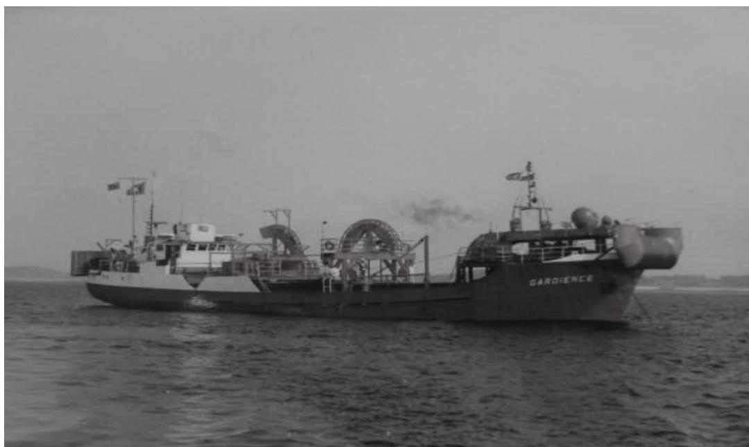
The vessel was converted into a cable layer by adding two large cable tanks in her hold, and a stern skid over which the cable was to be laid on the sea bed.
