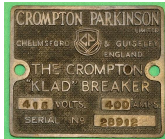
Fig. 5 Crompton Parkinson low voltage 'KLAD' circuit breaker
