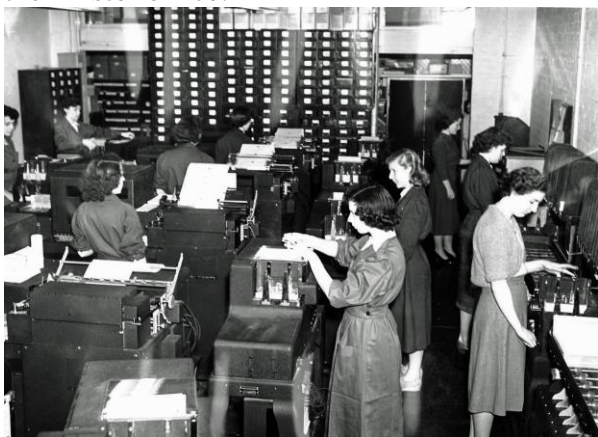
Fig. 2 Armada Street office with Hollerith Billing Machines
